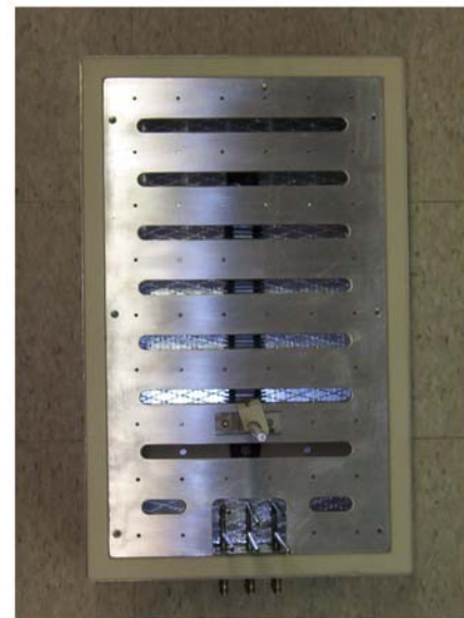
Figure 3-4 Photographs of instrumentation for controlled isothermal environment used for permeation experiments. Clockwise from top left: 1) base of instrument showing tubing bulkheads (front face) and aluminum base plate; 2) oven base with insulated top in place; 3) top view of oven base with base plate installed; and 4) top view of oven base with aluminum base plate removed to show finned heater and tubing.
