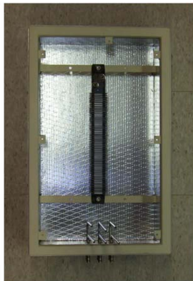
Figure 3-4 Photographs of instrumentation for controlled isothermal environment used for permeation experiments. Clockwise from top left: 1) base of instrument showing tubing bulkheads (front face) and aluminum base plate; 2) oven base with insulated top in place; 3) top view of oven base with base plate installed; and 4) top view of oven base with aluminum base plate removed to show finned heater and tubing.
